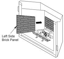
Figure 43 - Installing Side Brick Panels
